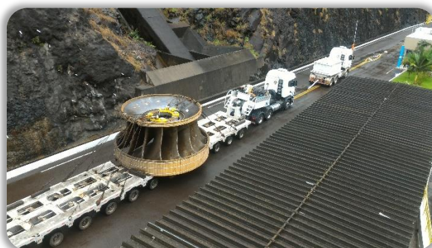
Arrival of Salto Osório HPP GU5 turbine rotor
